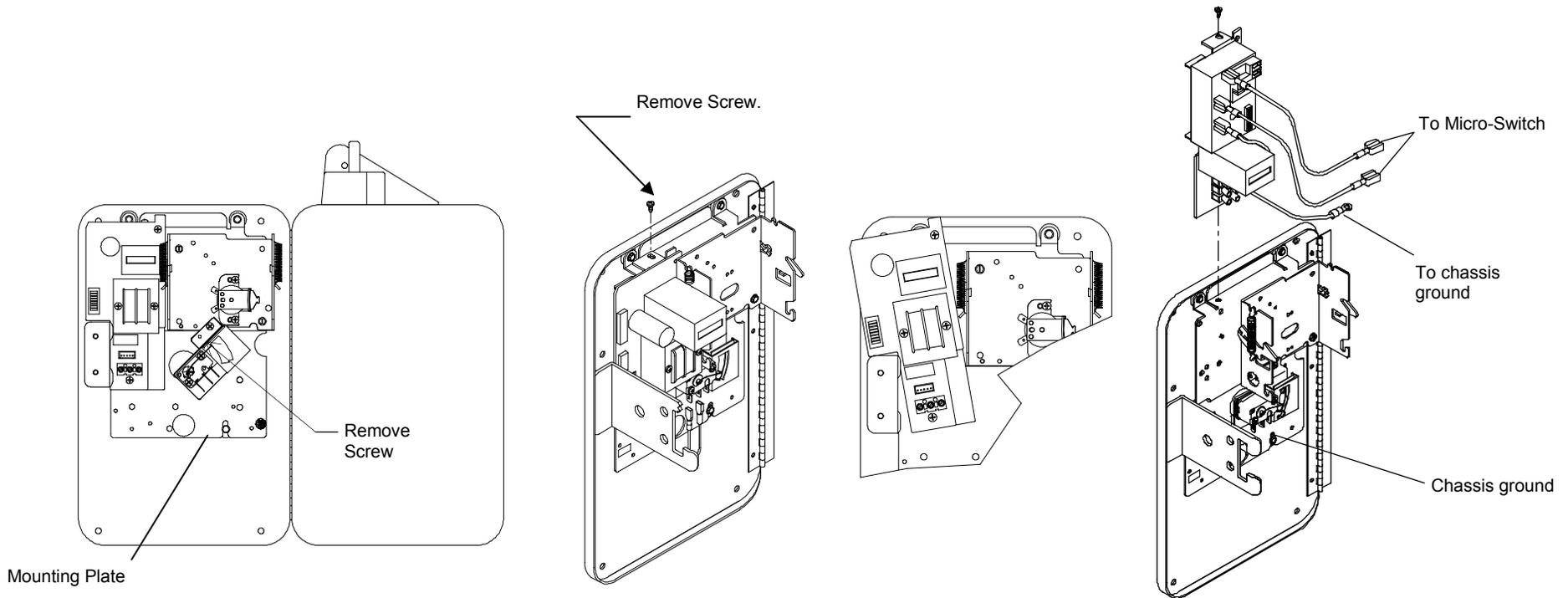
Remove left screw on switch bracket assembly and swing switch and bracket assembly out of the way To provide room for mounting new timer.
