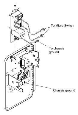
Remove left screw on switch bracket assembly and swing switch and bracket assembly out of the way To provide room for mounting new timer.
