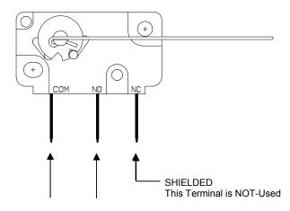
**CONNECT THE WIRES** FROM ATV-TIMER TO THE COIN MIRCO-SWITCH "COM" AND "NO" TERMINALS
